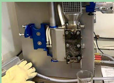
Melted at 200 degrees celsius at 25RPM dosage done by hand as well as extraction.
