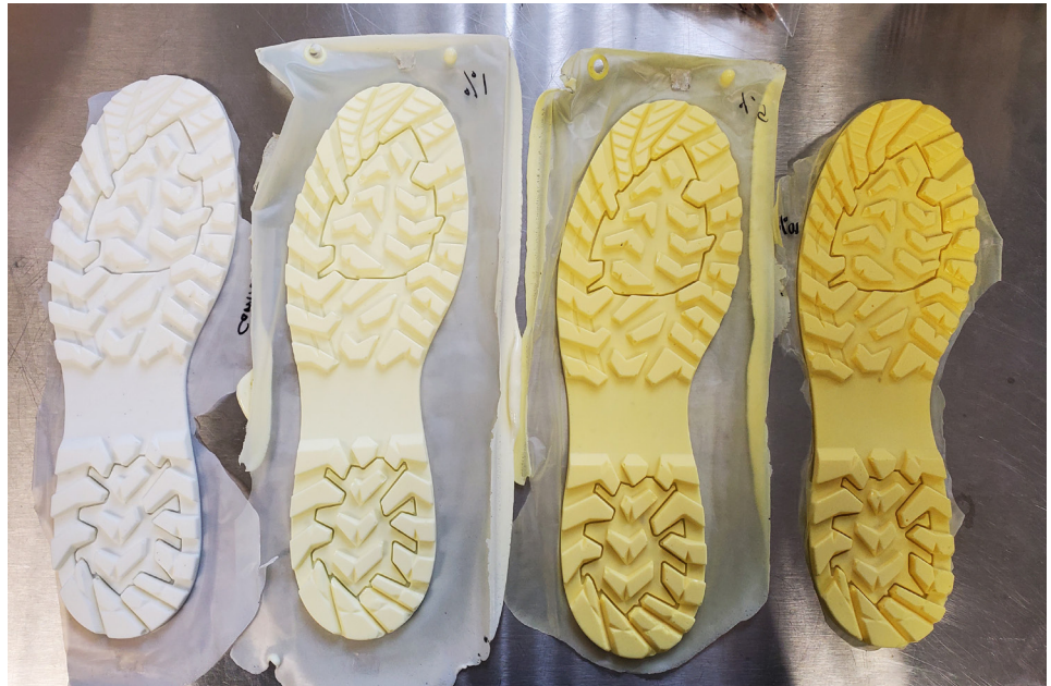
Synthesized PU outsoles with 0%, 1%, 5%, and 10% (left to right) dynamic monomer integrated are used to compare mechanical properties, recyclability and degradability between PU-vitrimerers and controls incapable of reprocessing.
