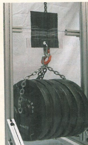
Geckskin: Displaying its power, Geckskin holds 300 pounds with only a 16 square inch adhesive pad.
